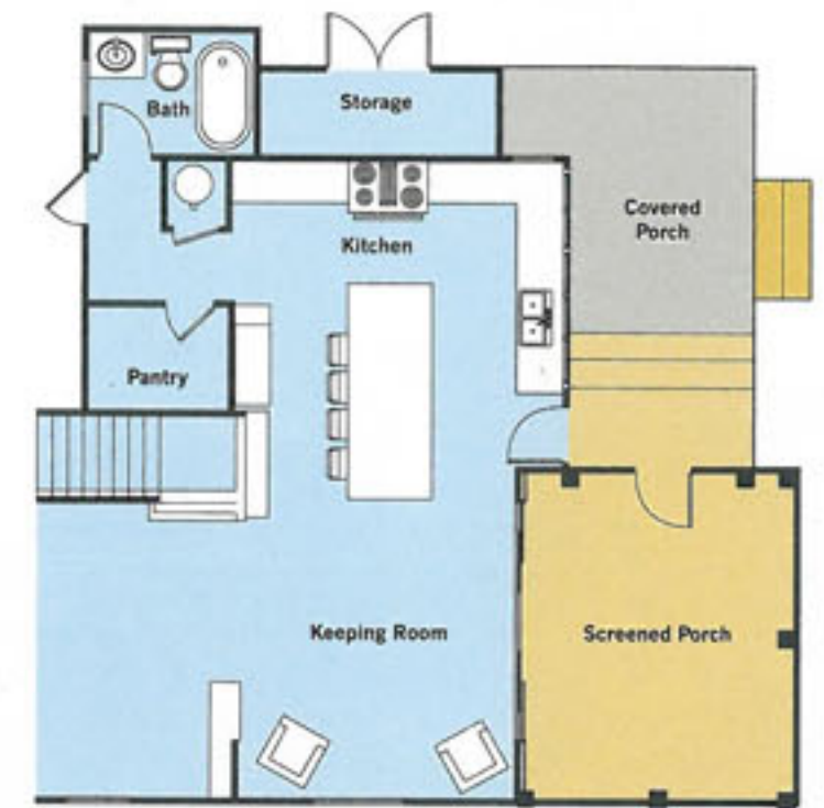
AFTER: A complete renovation reworked the back of the house, creating a single large kitchen with an open family room at one end and easy access to outdoor living areas through a new screened porch. Part of a bedroom became a walk-in pantry.
